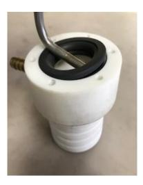
3. After seal is removed, wipe and clean out the inside of the housing.
