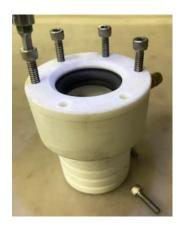
2. Use a screwdriver or similar tool to pry the old seal from the housing. Alternating sides will aide in the removal.
