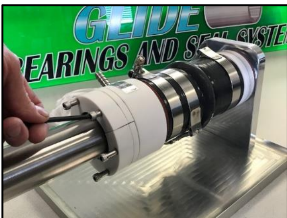
Figure 9 SECURE THE SCREWS USING AN ALTERNATING PATTERN TO EVENLY PRESS THE SEAL INTO THE HOUSING.
