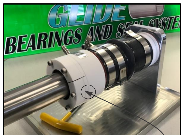
Figure 10 MAKE SURE THERE ARE NO VISIBLE GAPS BETWEEN ANY OF THE ASSEMBLED COMPONENTS.
