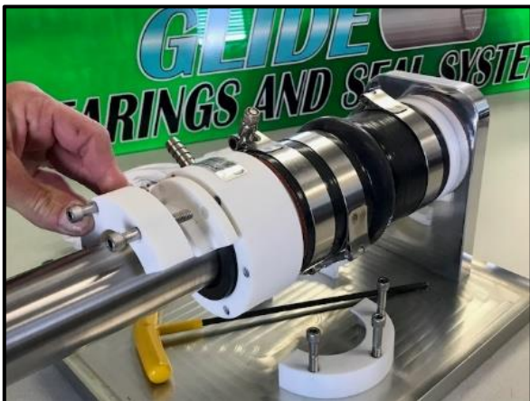
Figure 7 REINSTALL THE COVER AND PLATES TO THE HOUSING.
