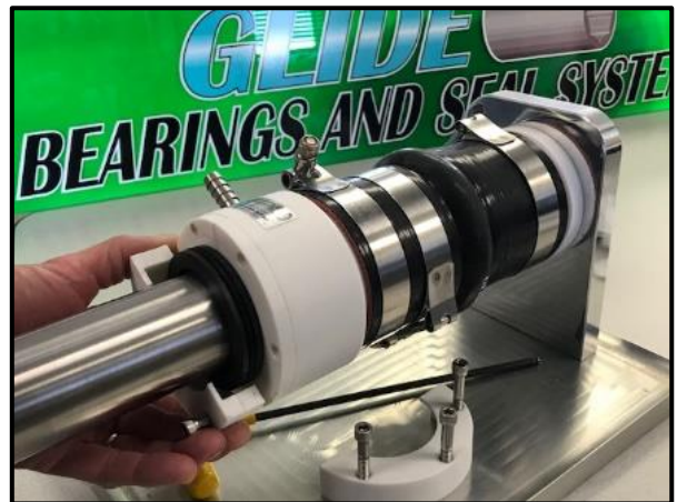
Figure 2 REMOVE THE SPARE SEAL COVERS AND SET ASIDE.
