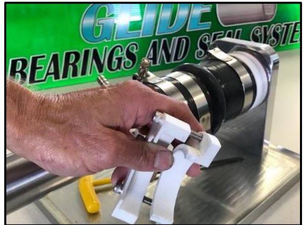
Figure 6 REVERSE THE PRESS PLATE LEG TO FIT INTO THE COVER (AS SHOWN). **BOTH PIECES MUST BE REINSTALLED**
