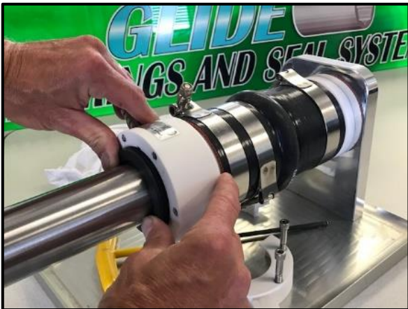
Figure 5 SLIDE SPARE SEAL INTO THE HOUSING. PRESS THE SEAL AS FAR AS POSSIBLE BY HAND.
