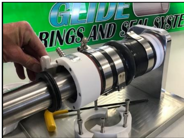
Figure 3 SLIDE THE SPARE SEAL FORWARD AND REMOVE THE PRESS PLATES.
