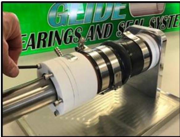
Figure 1 REMOVE THE 6 COVER SCREWS WITH THE PROVIDED WRENCH.
