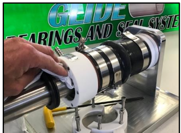
Figure 4 WIPE AND CLEAN THE SEAL HOUSING AND SHAFT AREA OF ANY DEBRIS.
